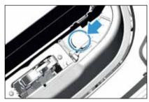
• Remove the tire inflator or the charger from the tool kit in the trunk and attach the power cable end to the car.
