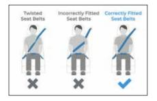
Each seat belt must be used by only one person. Never travel with a child sitting on the passenger's lap and a single belt to protect them both. In general, do not place any objects between the person and the belt.
