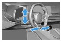
The steering wheel can be adjusted both in height and in depth.
