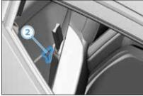
Install the child seat and pass the upper tether strap over the top of the seat back, under the head rest, secure it to the anchorage and tighten fully.
