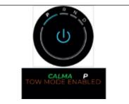
**Disabling Tow Mode:** with the vehicle powered on (i.e. visible by having the infotainment screens on), press the power button once. The electronic parking brake will be heard engaging and the notification about the Tow Mode Enabled on the center screen will no longer be shown. Vehicle will return to the vehicle awake but not engaged mode.
