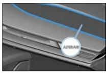
▲ WARNING: NEVER use a rearward facing child restraint on a seat protected by an ACTIVE AIRBAG in front of it, DEATH or SERIOUS INJURY to the CHILD can occur. ALWAYS comply with the instructions applied to the driver/passenger side sun visor as well as the label that is also placed on the roof headliner.
