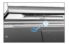
Glove box is equipped with a light source to provide additional visibility of interior compartment to the user. Light will turn on automatically when the glove box has been opened and will remain on for 30 seconds, after which it will turn off. If necessary, pressing the button again will further extend the duration of the glove box lighting another 30 seconds.
