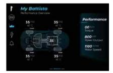
System may not show the pressures immediately if the vehicle has just been turned ON after an extended period of no driving activity. Some driving needs to take place before the values can be read back on the screen; this is considered normal as the sensors will go to sleep after some time of not detecting a tire revolution.
