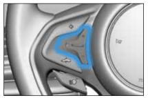
Cruise Control is an electronically controlled driving assistance system that allows the desired car speed to be maintained, without having to press the accelerator pedal.
