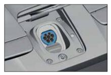
• Insert charging cable into the charging port socket firmly.
