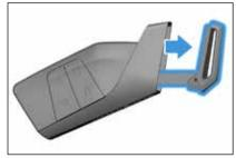
• Place the key in its cubby holder in the center console so it can be detected by the system to start the car.
