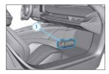
▲ WARNING: Follow the proper inspection intervals for the fire extinguisher – if the inspection intervals are not followed, functionality is no longer guaranteed. Check the pressure gauge, if the yellow pointer is in the red zone, the extinguisher is inoperable. The extinguisher should be checked by an authorized specialist every 1-2 years to ensure proper operation. **WARNING:** Follow the operating procedures on the fire extinguisher. Improper use could cause serious injury or damage.
