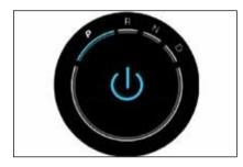
The gear selector knob is equipped with a rotary switch and a button. The center button is used to access functions of the vehicle like turning the powertrain ON and OFF, engaging and disengaging the Electronic Parking Brake (EPB).
