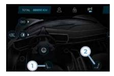
By touching the related arrows on the touchscreen, you can make seat adjustment to find your desired settings. To adjust lumbar settings, it is necessary to touch the related button to enter in the lumbar adjustment menu, by touching + or – buttons it is possible to find the desired setting.
