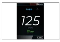
When your current speed is lower than 30km/h or above 250km/h and you request to activate Cruise Control, a speed limit notification appears on the center info display. The system will be automatically deactivated by pushing the brake pedal.
