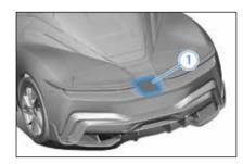
• Upon opening the charge port door, remove plug that covers up the connections within the port - NOTE this is only necessary if performing a DC charge, if AC charging keep the cap in place.
