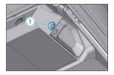
mechanical key blade. To reset the vehicle back on after accidental shut down, a button 1 in the trunk compartment is available on the passenger side which allows you to set the power back on by pressing it.
