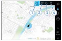
Once destination has been selected, the display shows you the turn-by-turn instructions to reach it. While driving the arrow down near street instruction displays the route overview showing when the next turns are expected during the currently selected route.
