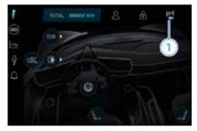
The camera feed will then be projected on the right screen, where the view can be toggled between each camera. If the speed exceeds 16km/h or 10MPH. the camera will not be selectable and a message indicating exceeded speed will appear.
