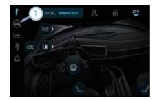
• NOTE Each Drive Mode screen represents the available driving characteristics of that mode, and it will allow you to alter the Mode to your preference. The Drive Mode screen will not allow the driver to select the desired Mode, this must be done using the door mounted knob. The following chart explains all the possible standard and optional characteristics of the four predefined driving modes.
