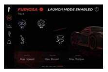
Drive mode is designed for driving on the racetrack in high grip conditions. Launch Control is available only in this mode, to obtain maximum performance. Possible customizations are: Regenerative braking (Low/ High), Steering (Sport/Standard), Suspension (Track/Sport) Stability Control (Sport/OFF).
