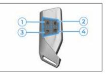
• NOTE Charge port door can be unlocked by pressing button 4 on the key fob for 3 seconds which will unlock the port door.
