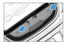
• Attach the power cord to the power port under the removed cover.
