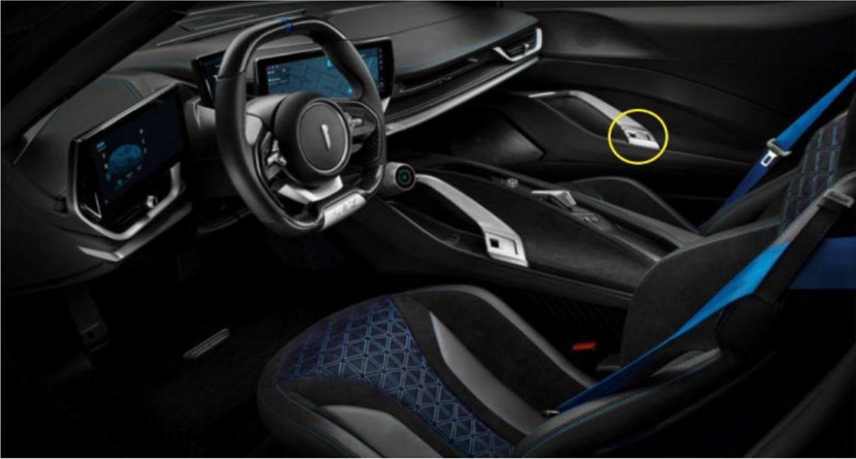
In case of an accident where the vehicle's power is disabled, the doors can still be opened from the inside.
